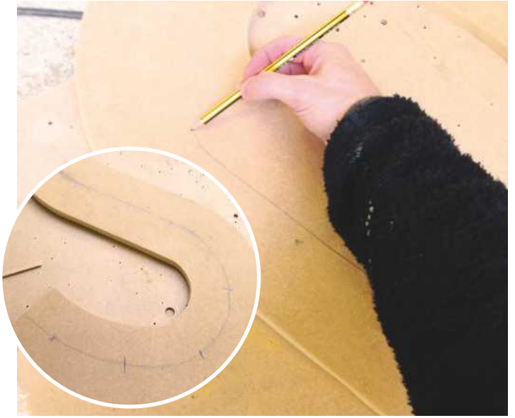
▲ Pic.5 The only part I hadn't designed on AutoCAD was where the holes for the bulbs would go. I just ran a pencil line round the centre of my 'S' then started to set out where the holes would be drilled. By my poor calculations, I figured out that for 10 bulbs, they would be every 150mm or so. At this point, I suggest double checking your measurements, as I made a stupid mistake here which I did not notice. See if you can spot it before I tell you in the next step!
